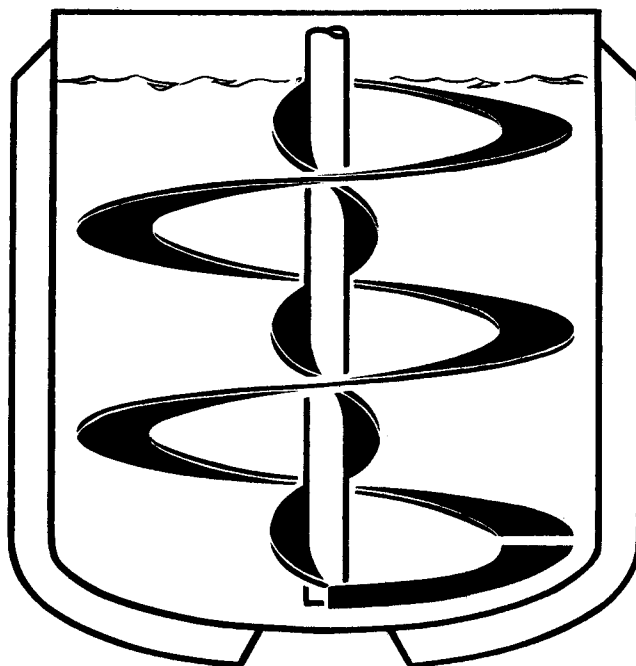
Fig. 1. A schematic view of a helical impeller in a jacketed tank.
